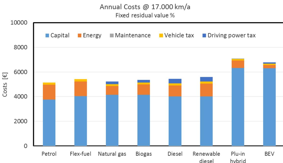
Figure 0.3: Annual cost with a fixed residual value and 17,000 km/a mileage.
