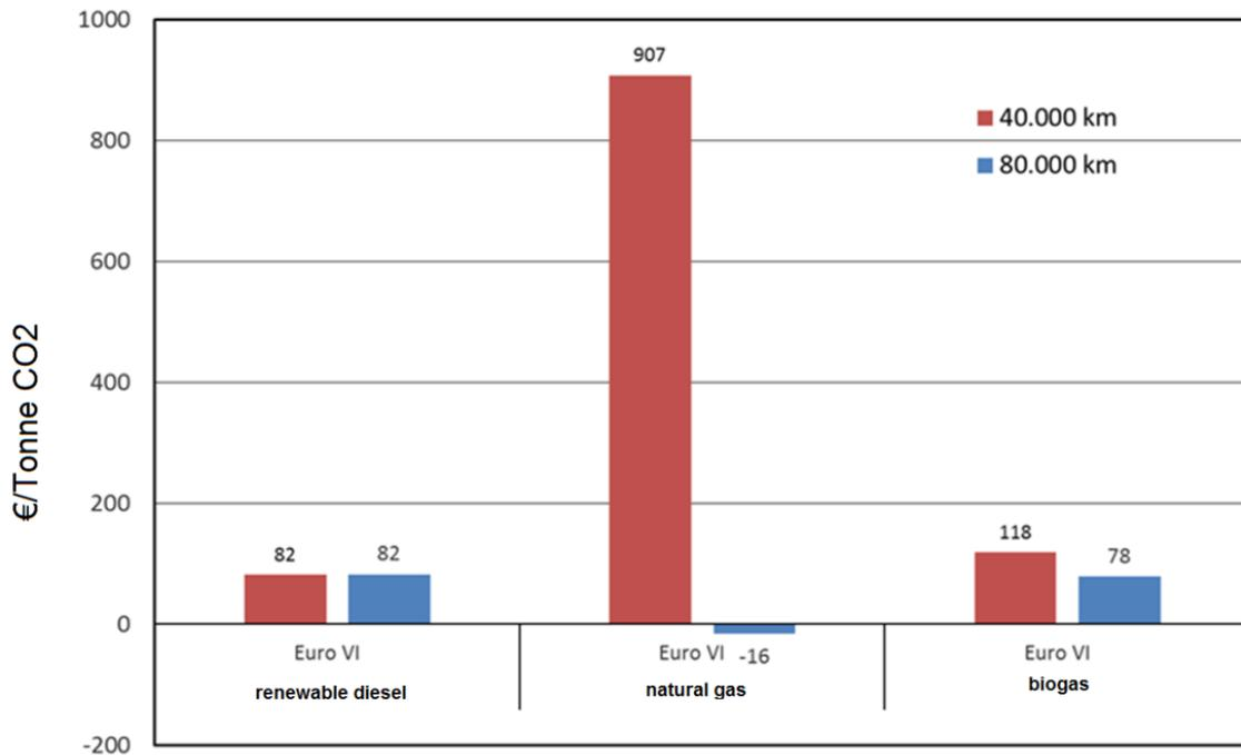
Figure 0.7. The cost of avoided CO<sub>2</sub> tonne for a bus with a typical annual mileage of 80,000 km as well as with an alternative mileage of 40,000 km/a.
