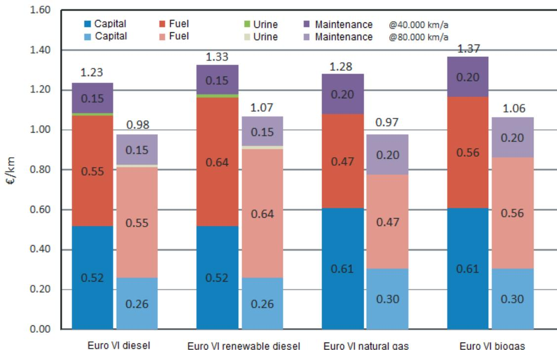
Figure 0.6: Costs per kilometre for buses, with different fuel alternatives. Mileages 40,000 or 80,000 km/a.
