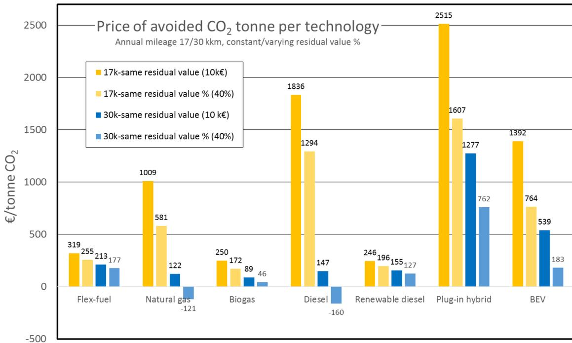
Figure 0.5: Cost of avoided CO<sub>2</sub> tonne with different residual values and mileages. A fossil fuel-based petrol vehicle was used as a point of reference.
