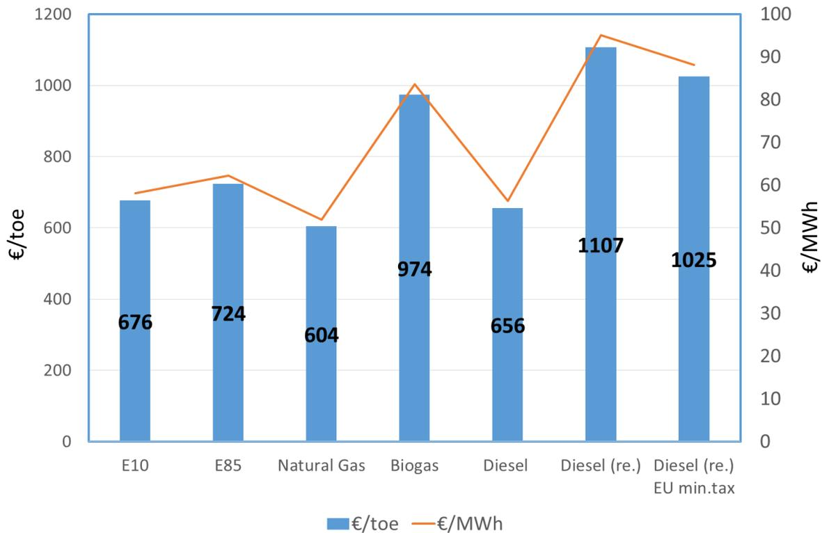
Figure 0.2: Tax-free pump prices of different fuels in proportion to energy content. Diesel (re.) stands for 100% renewable diesel. Compression to distribution pressure (200 bar) is included in gas prices.
